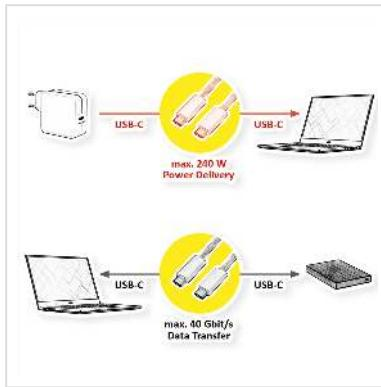
**USB4 Gen 3x2 Cable in very high quality with the reversible USB-C plug at both ends for data transfer rates of up to 40 Gbit/s and USB Power Delivery up to 48V / 5A (240 W). Cable jacket made of white textile braiding to perfectly fit the design of the Apple iPhone 15 products.**
