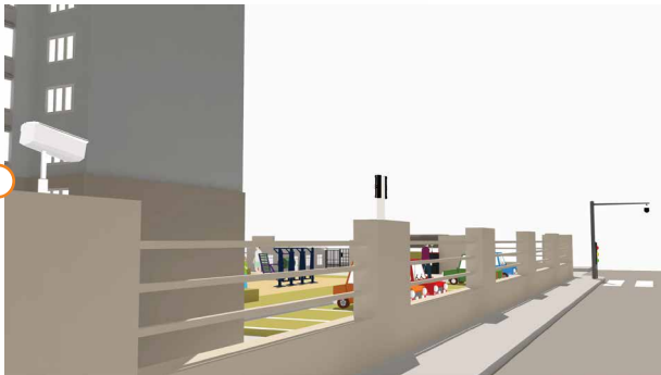
Fence Intrusion alarm CCTV surveillance
